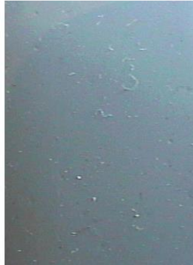
Gel Coat with Aerosil 200 + 30% BYK-R 605
