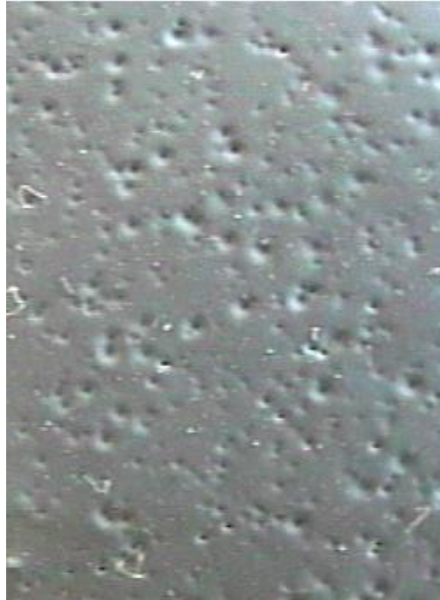
Gel Coat with Aerosil R 972
